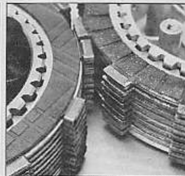
Suzuki factory racing clutch plates (left) feature paper fiber friction material and folded-over engagement tabs, which help absorb shock loads.
