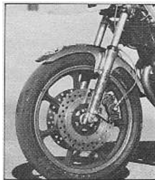
Forks are adjustable in four ways for almost infinite combinations. Discs are drilled stockers with Lockheed calipers.
