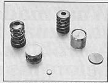
Race bike uses Yoshimura buckets with small shim located underneath, versus large shim on top of stock bucket.
