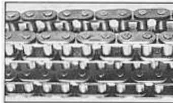
Cam chain has one more link than stock. Outside run is polished to reduce wear on tensioner slippers.
